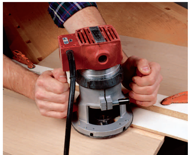
Figure 2: To make this straightedge jig, fasten a straight, narrow board to an oversized piece of hardboard, then rout the edge of the jig with the router and bit you intend to use for the dado. Next, align and clamp the edge of the jig with the layout line and rout the dado.
