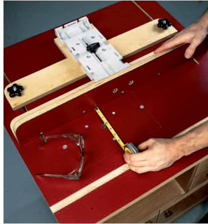
Our router table is full of convenient features that make it a more efficient shop tool. Ample storage space in the drawers and cupboard provides room for routers, bits and other accessories; the interchangeable insert plates accommodate a wide range of router bit sizes; and the fence system adjusts mechanically or the old-fashioned way—with a quick tap of the hand at one end.
