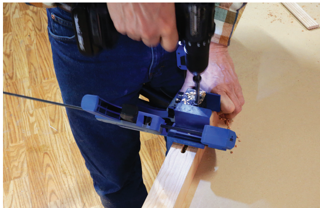
Photo 5: Mark a line 1½" down from the top of each leg on two adjacent faces. Prepare the Beadlock with two spacers and the 3/8" drill guide set in the "A" position. Bore three holes to their proper depth (see Sidebar).
