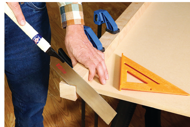
Photo 1: Square the end of the leg stock. Draw a line around three edges and cut along those lines. Start as shown in the photo, then rock the saw back along the top line. Be careful to keep the saw on the marked lines.
