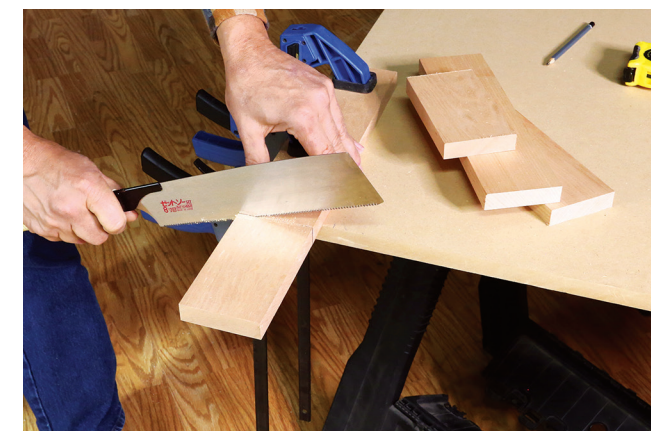
Photo 4: The Material List (below) also provides the length for the long and short aprons. Each piece must have square-cut ends to fit properly.
