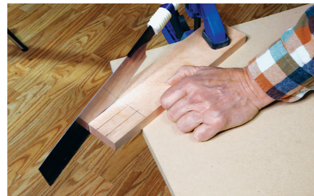
Photo 13: Mark the piece of leftover stock, as shown in the photo above. Saw down each of the long lines. Cut across the piece to free the four glue blocks. The exact size of these pieces is not critical.
