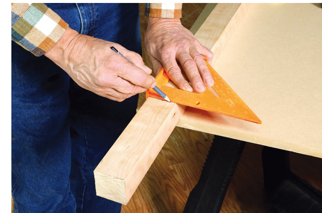
Photo 2: Mark the squared-up leg stock to the length of the legs found in the Material List. It specifies the length of each piece. The width and thickness of this stool's parts are determined in the dimensioned stock.
