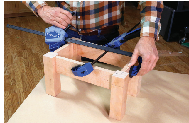
Photo 9: Clamp all the parts together, but without glue, to make sure that all the pieces fit together well. Take the pieces apart. The Beadlock tenons may be difficult to remove; you may need a pliers to get them out.
