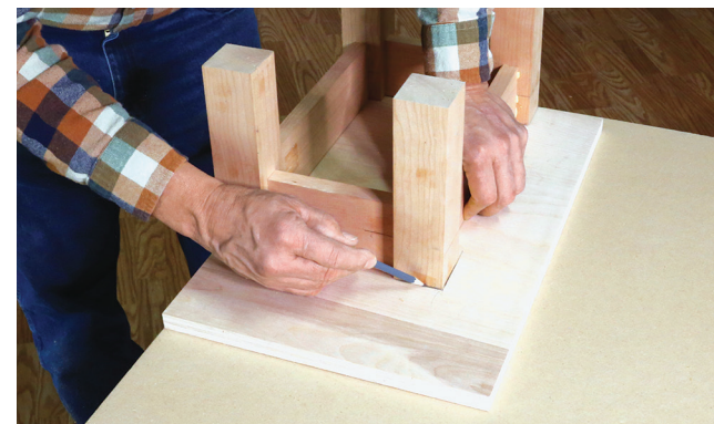
Photo 11: Place the leg/apron subassembly on a piece of plywood and mark its shape. Extend those lines to draw the rectangular shape of the top. This is the one piece that may differ a bit from the Material List.
