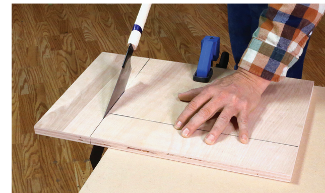
Photo 12: Cut the top to shape, following the marked-out lines carefully. Then sand the edges of the top to remove any splinters and smooth the edges of the plywood. Fill any edge voids with wood putty.
