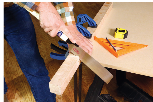
Photo 3: Use the same technique shown in photo 1 to cut off the first leg. It is important to keep each cut square. Make the other three legs.
