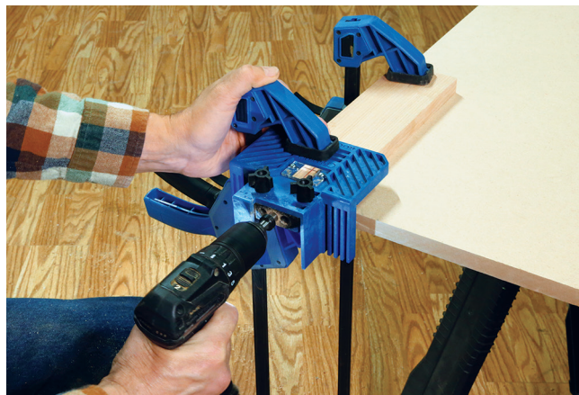
Photo 8: Remove the spacers from the Beadlock jig and remount the drill guide. It is sized correctly to center the mortises in 3/4"-thick stock such as these aprons. Align the jig to a line marked 1½" from the edge.
